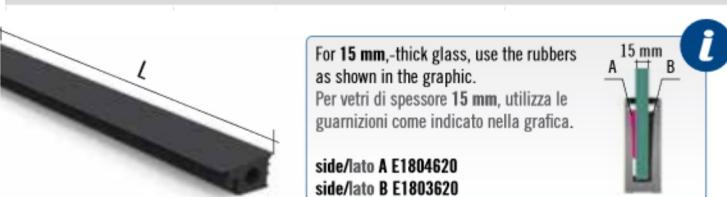
For 15 mm-thick glass, use the rubbers as shown in the graphic.
